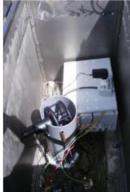
Vertical profiles of \text{CO}_2 in boreholes (left) and air control station at point 4 with data-logger and probes of temperature, humidity, \text{CO}_2 , direction and speed of air (right).
