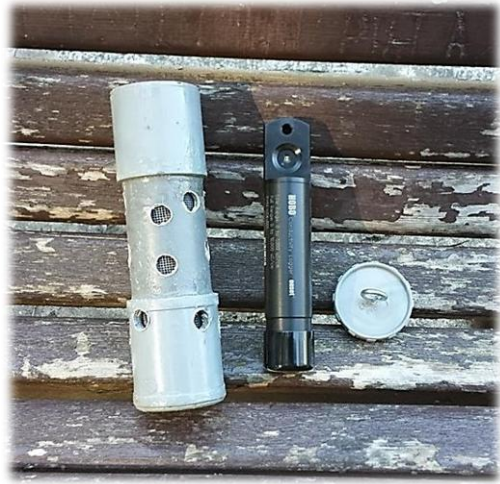
Conductivity and temperature sensor for continuous monitoring
