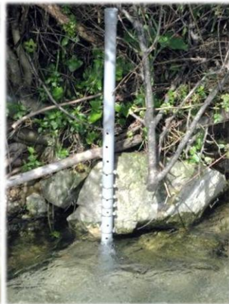
Capacitance water level probe for continuous flow discharge monitoring
