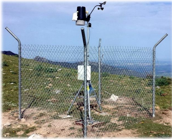
Weather station recently installed in Grazalema area to monitor rainfall
